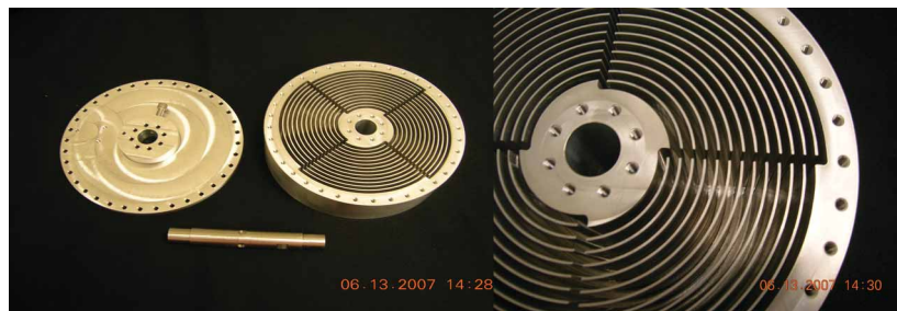
Figure 1. Photograph of the spiral tube support. Multiple spiral layers can be made from one piece of plastic tubing. Material: aluminum; dimensions, 18 cm in diameter and 5 cm in height; grooves, 4 spiral grooves and 4 radial paths all 4.8 cm deep each 2.8 mm wide, each spiral groove can accommodate about 1 m of tubing.
